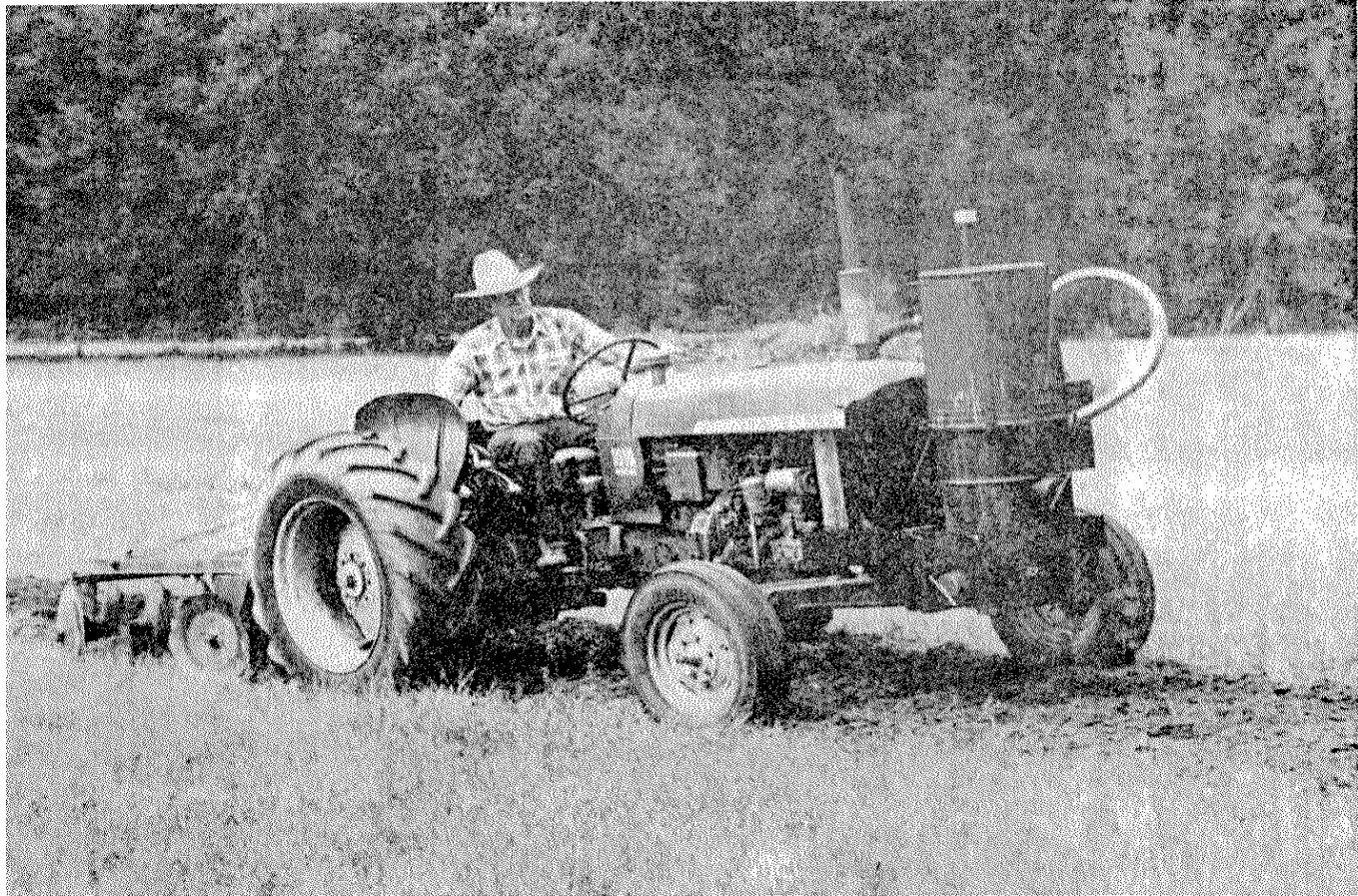
Fig. S-3. Wood gas generator unit in operation during field testing.
